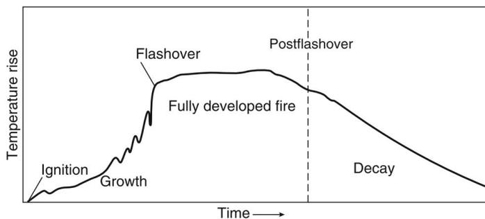
Figure 1 – Generic illustration of fire development in a room expressed by the temperature development [6]
